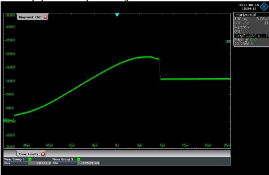
Oscilloscope picture of fast pulses during switch off 12 VDC:
