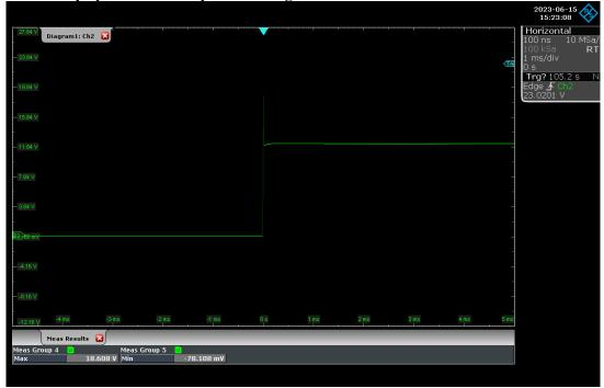
Oscilloscope picture of slow pulses during switch off 12 VDC:
